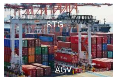
自働搬送台車(AGV)と遠隔自働 RTG
