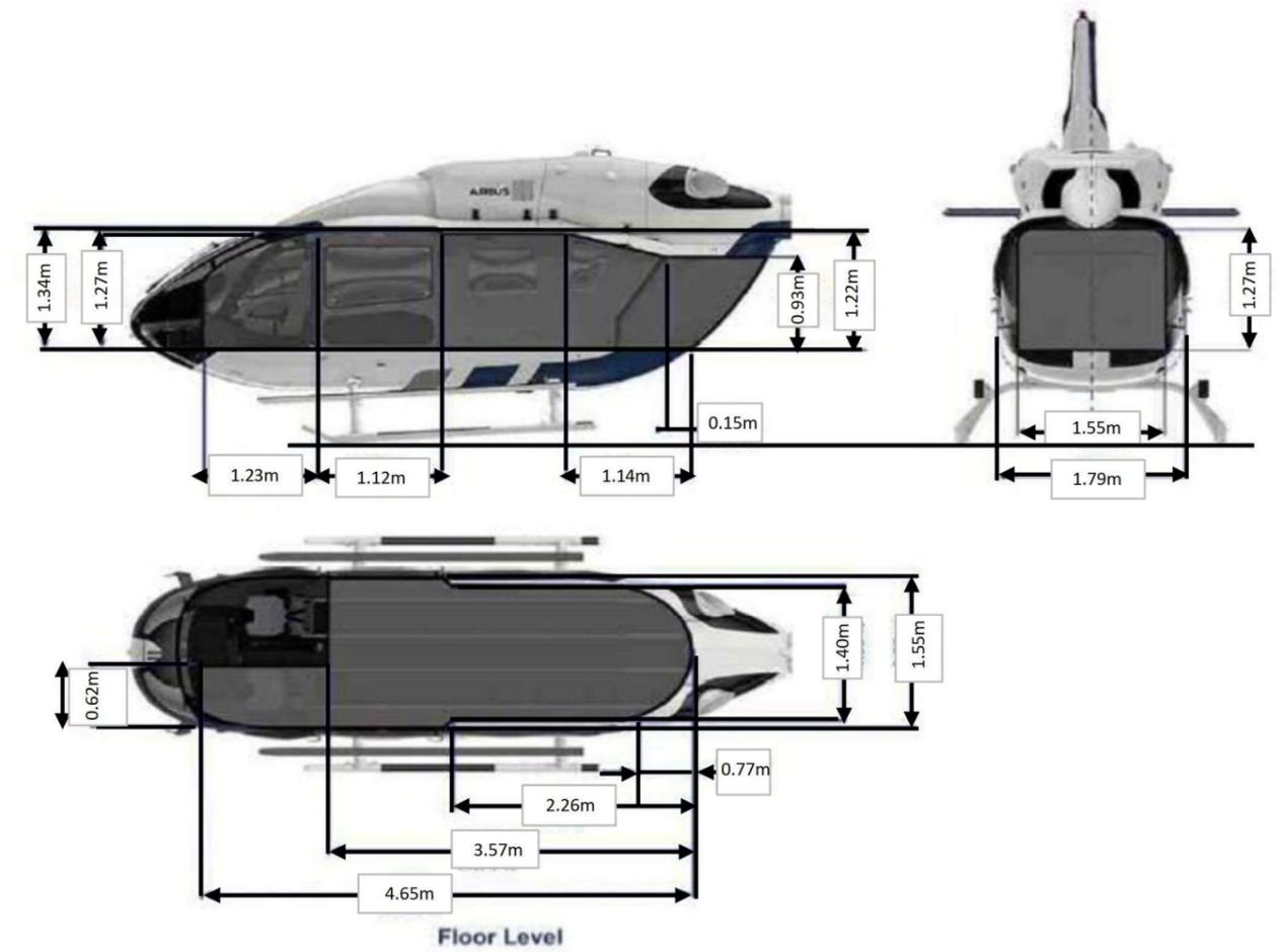
Figure 2.3: Internal dimensions
